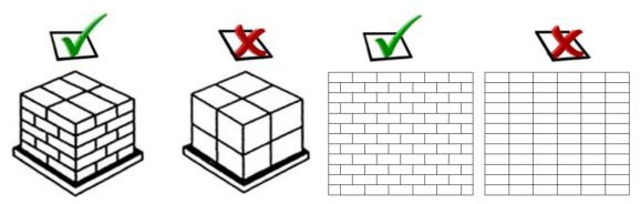
• Below is another example of how to brick stack goods to interlock the load and avoid collapsing. The direction of stacking alternates from vertical to horizontal every two layers. The pressure of the upper layer on the lower can be better distributed with intermediate layers of strong cardboard or dunnage.
